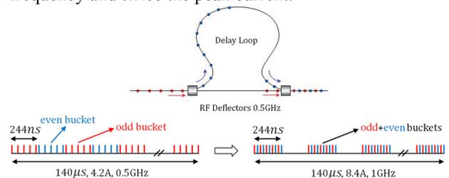
Figure 4: The principle of bunch combination in the delay loop [1].
