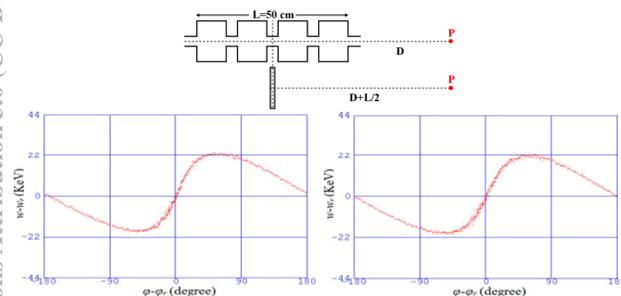
Figure 11: The phase space of the thin lens SHB (left diagram) and travelling wave SHB (right diagram).
