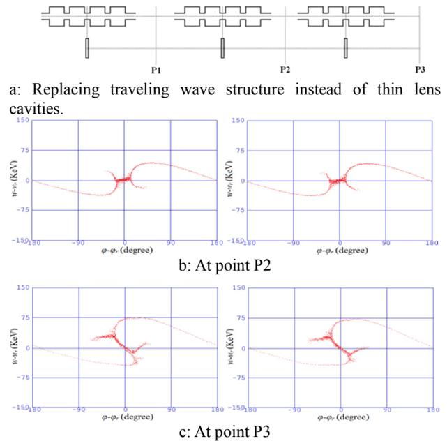
Figure 12: Comparison between thin lens system (left diagram) and travelling wave structure (right diagram) comparison at point P1 is given in Fig. 11.
