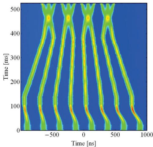
Figure 3: RF gymnastic for the production of the BCMS scheme at intermediate energy. The batch compression is followed by a bunch merging and a triple splitting.
