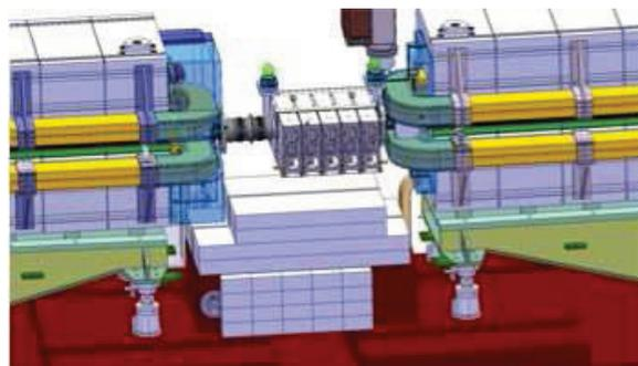
Figure 2: Finemet® cavities as to be installed in a PS straight section. The shielding blocks below the cavities protect the solid-state amplifiers from radiation.
