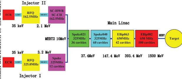
Figure 4: Layout of the C-ADS driver accelerator.
