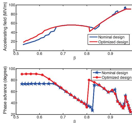
Figure 3: Comparison between baseline design and optimized design.
