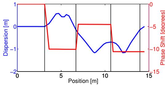
Figure 2: Phase feedforward optics dispersion and phase shift with the maximal kick. Vertical lines mark the positions of dipoles in the correction chicane.
