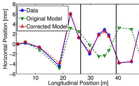
Figure 3: Optics kick measurements before and after applying corrections to the MADX model of TL2. Vertical lines mark the region of the TL2 chicane.
