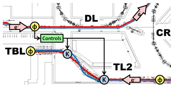
Figure 1: Simplified schematic of the phase feedforward system. Red and blue lines depict orbits for bunches arriving late and early at the first phase monitor,  $\phi$ , respectively. The trajectory through the TL2 chicane is changed using two kickers,  $K$ .
