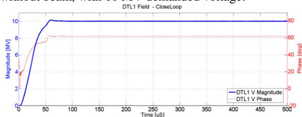
Figure 3: Magnitude and phase of DTL1 field. No beam.
