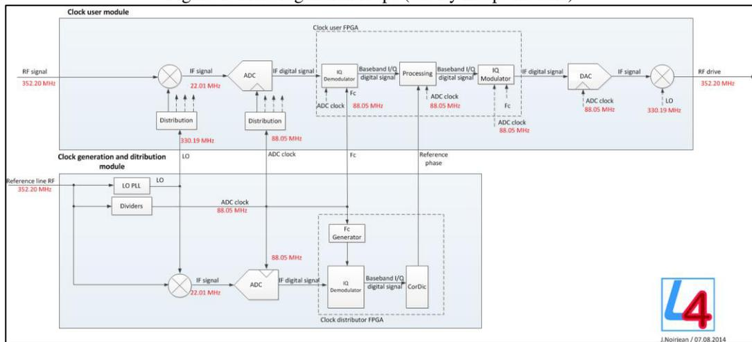
Figure 2: Demodulation, processing and modulation.
