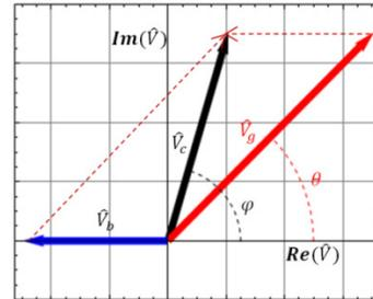
Figure 1: superposition of different cavity voltages in Complex plane as phasors.
