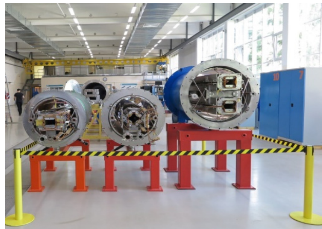
Figure 6: Serial dipole magnet and quadrupole lens doublet for Booster and preserial “twin” dipole magnet for Collider Full energy range two parts of energy range.
