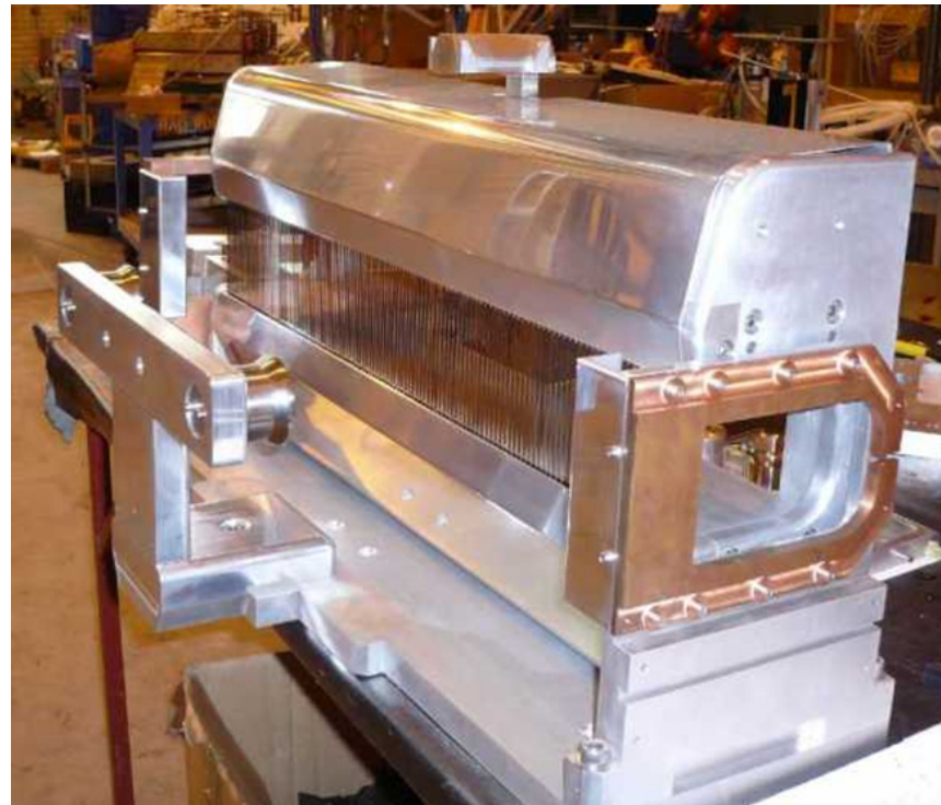
Beam splitter at iThemba
