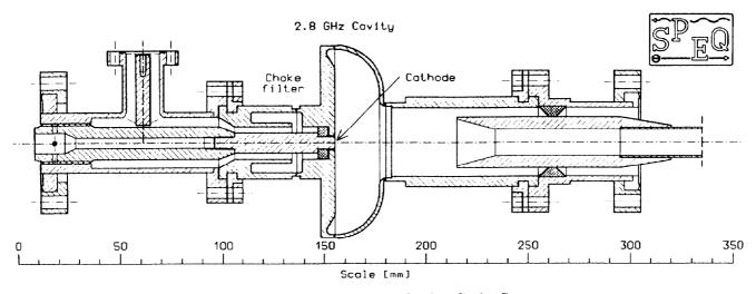
Figure 1: 2.834 GHz Superconducting Cavity Setup
