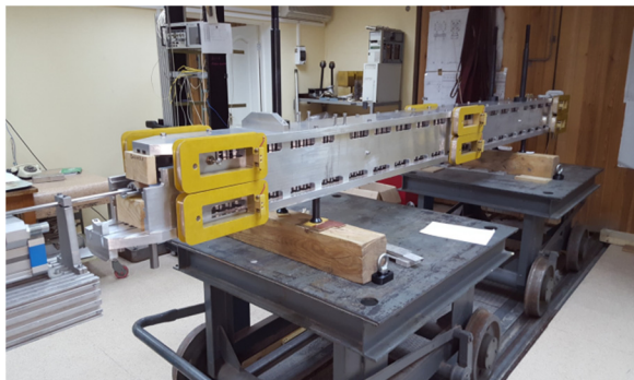
Figure 11. Variable Period Undulator \lambda_u=4.8-9.6 cm
