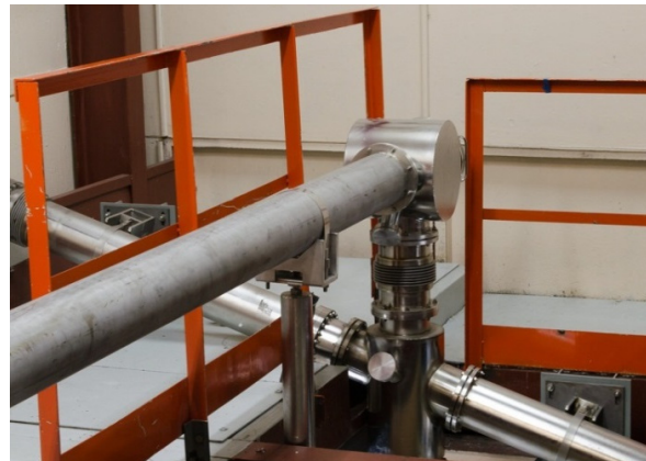
Figure 6. Optical beamline for FELs. Radiation of all FELs is delivered to the same user stations.
