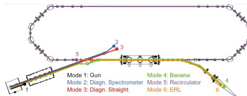
Figure 1: Basic bERLinPro layout and planned operation modes.
