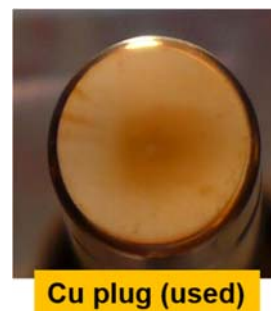
Figure 2: The copper cathode after used in the SRF gun II. A radius of 0.3mm is used to reduce the field enhancement on the sharp edge. The pattern on surface is believed from the flash during the rf commissioning.
