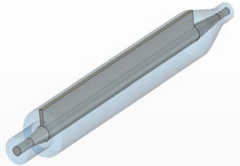
Figure 1: Schematic view of CSWG connected with coaxial lines at both ends.
