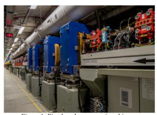
Figure 1: First bunch compression chicane.
