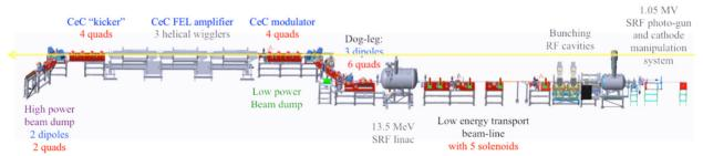
Figure 1: The layout of CeC experiment.
