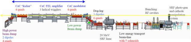
Figure 1: Layout of the proof of CeC principle experiment at RHIC IP2.
