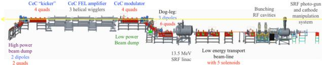
Figure 1: Layout of the CeC proof-of-principle system at IP2 of RHIC.
