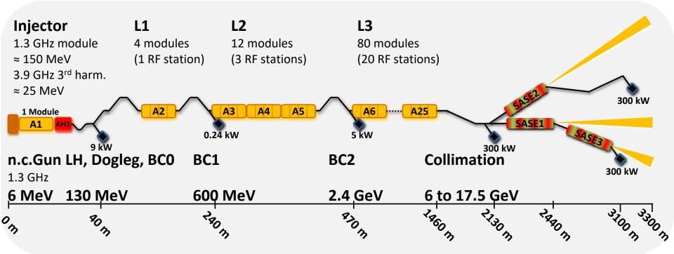
s.c. linac with 97 1.3 GHz superconducting modules + 1 third harmonic module
