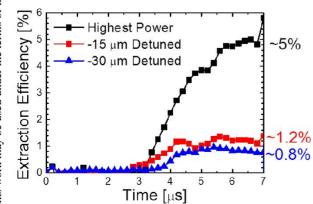
Figure 2: Temporal evolution of extraction efficiency under the relative cavity length of 0, -15 and -30  $\mu$ m. [15]
