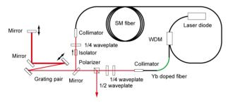
Figure 4: Schematic drawing of a fiber oscillator developed for a mid-IR seed laser. Output laser pulses are delivered to an amplifier followed by a difference frequency generation.
