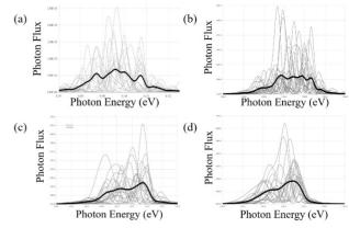
Figure 10: FEL spectrum of (a) 35 MeV, K 2.0, 26.47 THz, bandwidth 0.605 THz (b) 25 MeV, K 1.6, 17.77 THz, bandwidth 0.484 THz (c) 35 MeV K 3.321, 12.16 THz, bandwidth 0.362 THz (d) 25 MeV, K 3.321, 6.17 THz, bandwidth 0.254 THz.
