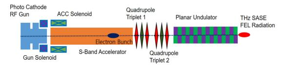
Figure 1: Schematic structure of THz FEL facility in PAL XFEL.
