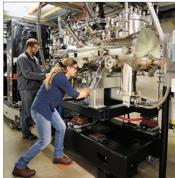
Figure 2: Helical SCU installed in Sector 7.
