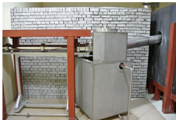
Figure 5: Target transport system in the target room.
