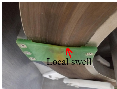
Figure 10: Local damage of type B MA core.
