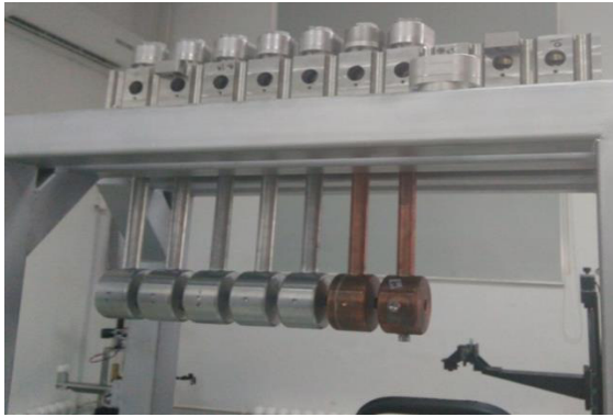
Figure 5: Alignment experiment with the test drift tubes.
