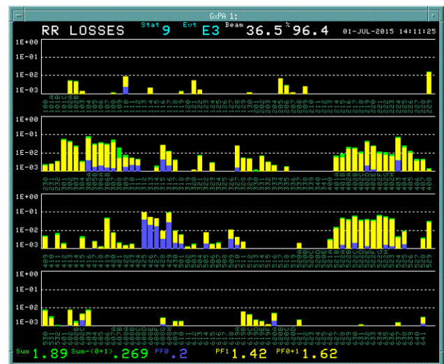
Figure 4: Loss around Recycler for 525 kW operation July 2015.
