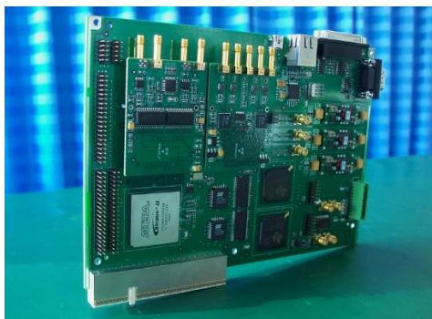
Figure 6: Digital feedback control board.
