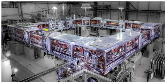
Figure 1: The cryogenic storage ring CSR with 35 m circumference.
