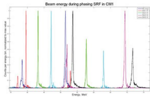
Figure 12: RF cavity phasing.
