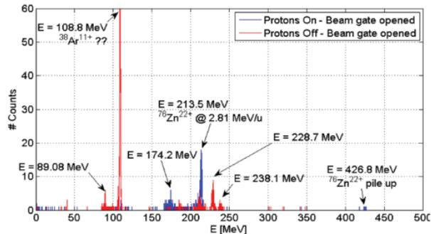
Figure 11: Particle energy spectrum.
