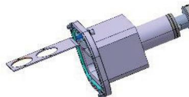
Figure 9: 3D model of a stripping foil mechanism.
