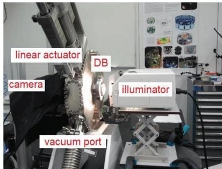
Figure 6: Scanning slit acceptance test set up [3].
