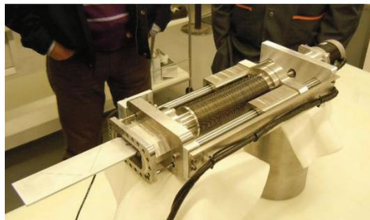
Figure 5: A scanning slit fully assembled.
