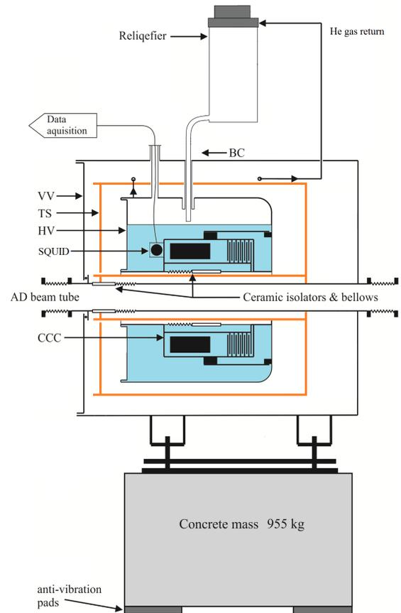
Figure 3: CCC cryostat schematic.
