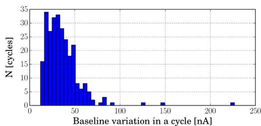
Figure 7: Distribution of the baseline drift for 271 acquired cycles where no beam was injected.
