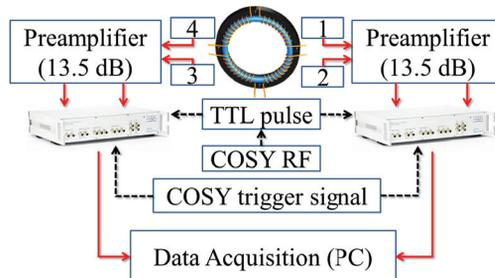
Figure 3: Readout scheme for the signals of one Rogowski coil BPM.
