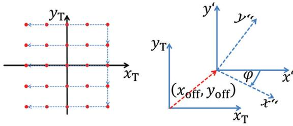
Figure 4: Left: coordinate system of the piezo table system. The dots show schematically the applied grid positions. Right: sketch of the coordinate system of the piezo table ( $x_T, y_T$ ) and the coordinate system ( $x'', y''$ ) of the Rogowski coil BPM, which is rotated with respect to the electrical centre by the angle  $\varphi$ .  $x_{\text{off}}$  and  $y_{\text{off}}$  define the offset to the electrical centre ( $x', y'$ ).
