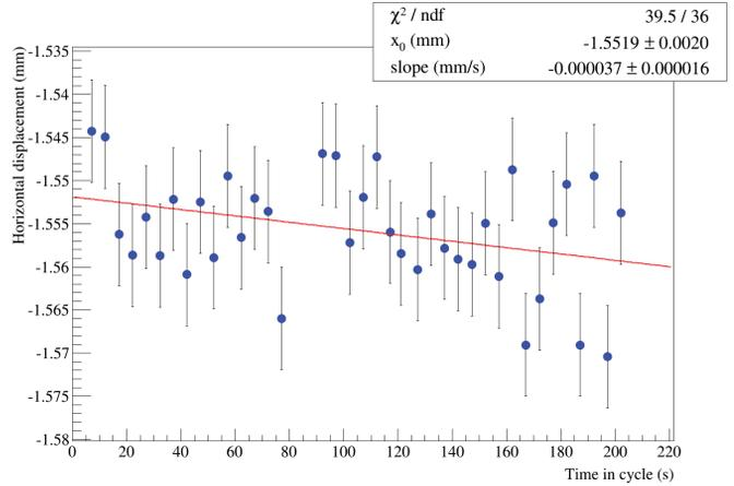
Figure 5: Corrected horizontal beam position. A linear fit is applied to determine the mean position of the cycle. The slope reflects possible drifts of the beam position during the cycle.
