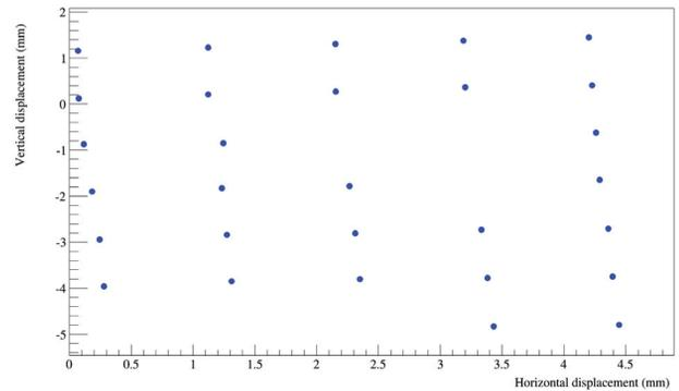
Figure 6: Measured beam position without calibration factors.
