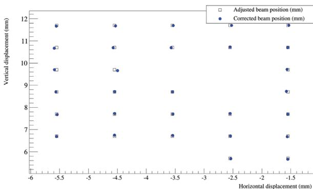
Figure 7: Corrected beam position with respect to the applied piezo table positions.
