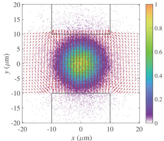
Figure 5: Transverse particle density distribution (color coded) from ASTRA simulation and transverse electric field distribution (red arrows) from CST simulation at the entrance of the SRR gap. The geometry of the gap is indicated by the black lines.
