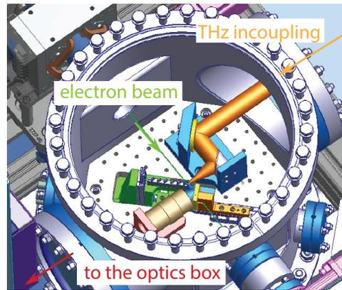
Figure 3: Technical drawing of the vacuum chamber.
