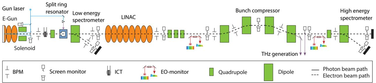
Figure 2: Schematic layout of FLUTE including various diagnostics elements. The proof-of-principle experiment for the SRR diagnostics is located upstream of the low energy spectrometer. Not to scale.
