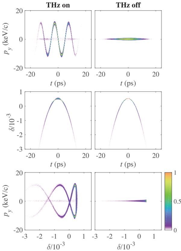
Figure 6: Particle distribution at the exit of the SRR structure with the THz deflecting field switched on (left column) and off (right column). The color code corresponds to the particle density.
