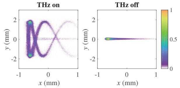
Figure 8: Simulated image of the electron bunch on the screen in the dispersive section. The color code corresponds to the image intensity.
