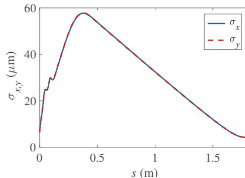
Figure 4: Transverse rms beam sizes from the cathode to the entrance of the SRR structure.
