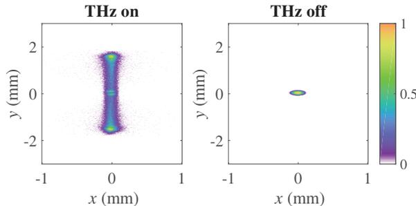
Figure 7: Simulated image of the electron bunch on the screen in the straight section. The color code corresponds to the image intensity.
