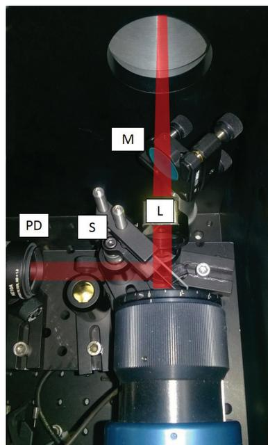
Figure 4: Controllable optics overlaid by the expanded laser beam that is focused by a 500 m lens (L) towards the IP with the  $H^-$  beam. An AR-coated beam sampler (S) diverts a 4% reflection to the photodiode.
