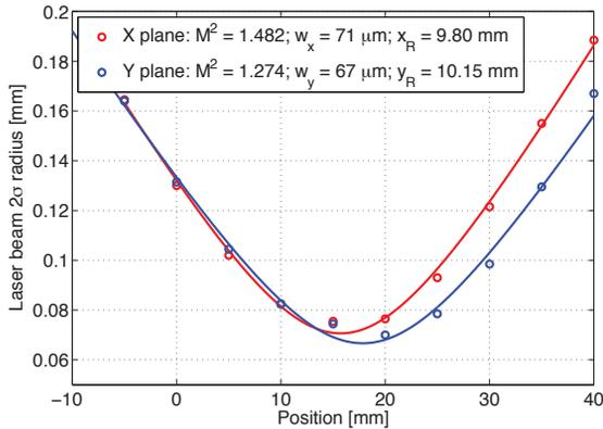
Figure 5: Spatial characteristics of the laser beam at the interaction point with  $H^-$ .
