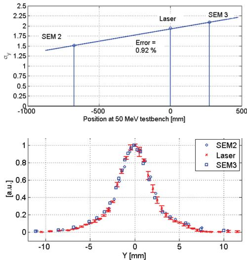
Figure 9: The vertical size of the 50 MeV  $H^-$  beam was measured using SEM grids and the laserwire. The laserwire profile is overlaid with profiles from the SEM grids scaled to the laserwire position.
