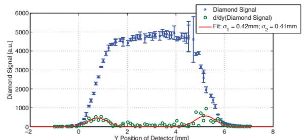
Figure 8: A fine scan of vertical detector position. The vertical beamlet size is extracted from the signal derivative.
