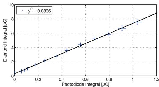
Figure 6: Integral of pulse signals recorded with the diamond detector versus the photodiode before the IP with the 50 MeV  $H^-$  beam.
