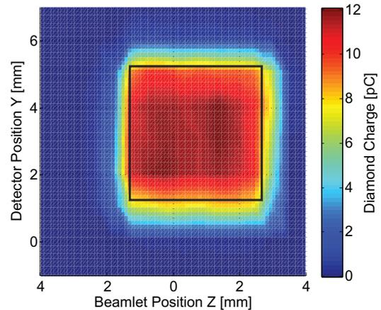
Figure 7: Integrated charge recorded during a two-dimensional scan of the diamond detector and inferred horizontal position of the beamlet. The black frame indicates the  $4\text{ mm} \times 4\text{ mm}$  surface of the diamond sensor.
