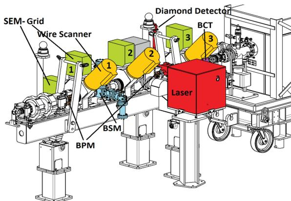
Figure 2: Diagnostics test bench used for LINAC4 commissioning of 50 MeV, 80 MeV and 107 MeV  $H^-$  beam [5].
