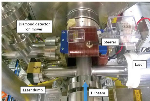
Figure 3: Vacuum-chamber for laser interaction and steerer magnet to deflect electrons towards the diamond detector [4].
