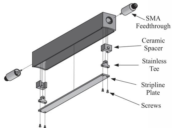
Figure 5: Exploded view of the single stripline detector.
