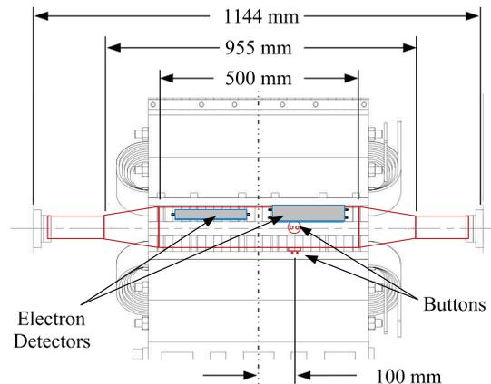
Figure 2: Detector chamber within the quadrupole magnet.
