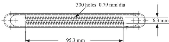
Figure 4: Holes are made in stainless steel plates which are then spot welded into slots in the beam-pipe wall.
