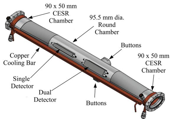
Figure 1: The detector chamber with electron detectors and the button electrodes used for microwave measurements.
