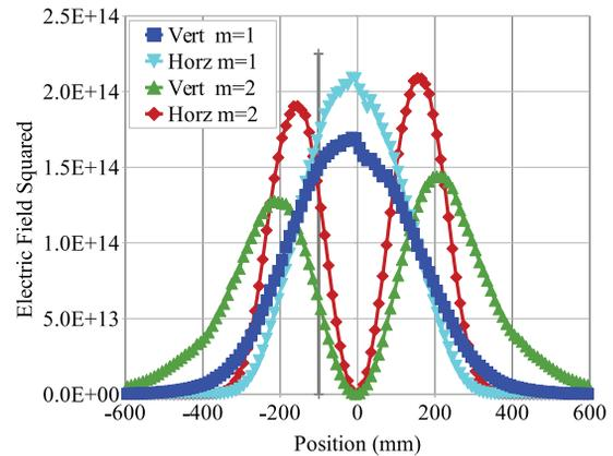
Figure 6: The results of a Microwave Studio<sup>®</sup> simulation show that the resonant microwave fields of the lowest four modes are contained within the 560-mm-long quadrupole magnet. Zero is the longitudinal center of the quadrupole.
