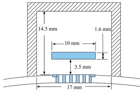
Figure 3: An array of small holes allows electrons to enter the detector vacuum space and be collected on the stripline.
