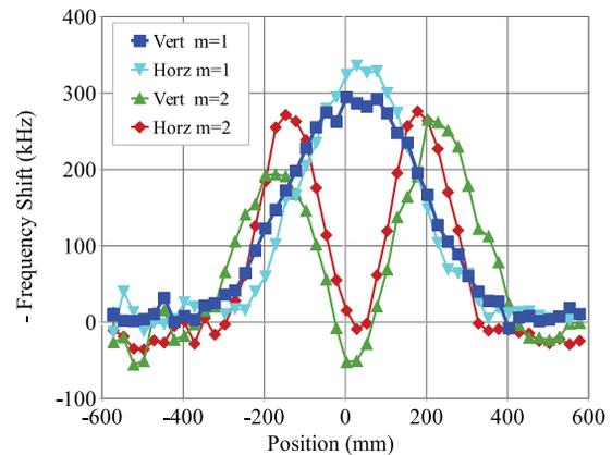
Figure 7: Beadpull measurements of the first two horizontal and first two vertical modes of the completed chamber.
