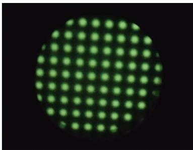
Figure 9: Light pattern imaged by MCP.
