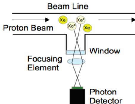
Figure 1: Schematic diagram of BIF monitor.
