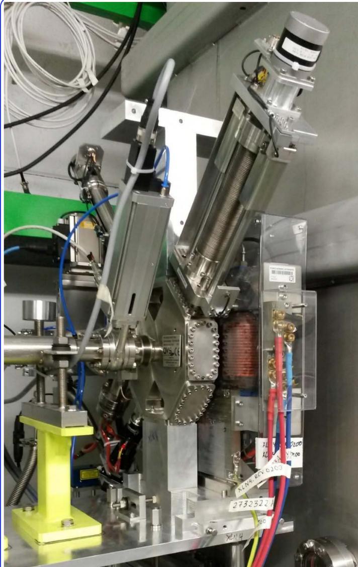
Figure 1: a short DB installed in the HIE ISOLDE LINAC
