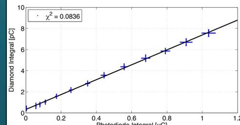
The diamond detector response is found to linearly follow the photodiode for a range of pulse energies. A small offset is observed due to a background of stray protons, H<sup>0</sup> or H<sup>-</sup> directly impacting the diamond sensor in the 50 MeV setup.
