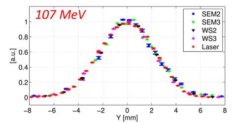
The vertical size of the H<sup>-</sup> beam,  $\sigma_y$ , was measured by laserwire scans at three beam energies and compared with measurements from nearby SEM-grids and wire scanners. Accounting for H<sup>-</sup> beam drift, the laserwire result is extremely close to the interpolated value between SEM-grids. The SEM-grid and wire scanner profiles are scaled to the position of the laserwire: **good agreement was found that is consistently below ±2% error on the H<sup>-</sup> beam size.**
