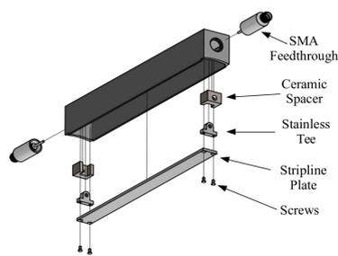
An exploded view of the single stripline detector
