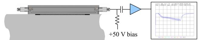
For data taking, the stripline signals are amplified and connected to an oscilloscope.
