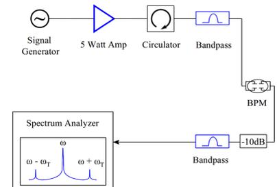
A train of bunches in a storage ring will produce a periodic electron cloud (EC) density. If the beam-pipe is resonantly excited with microwaves, the resonant frequency will be modulated by the EC density. The magnitude of the EC density can then be measured through the resulting phase modulation sidebands in the resonant response. In the sketch above,  $\omega$  is the drive frequency and  $\omega_r$  the revolution frequency.
