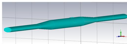
The round chamber with transitions to quasi-rectangular CESR beam-pipe was modeled in Autodesk Inventor<sup>®</sup>. The model was then imported to CST Microwave Studio<sup>®</sup> for simulation of the TE<sub>11</sub> eigenmodes.
