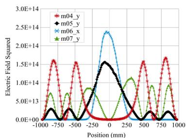
Simulation of a chamber with a 89 mm dia. round center section showed that most TE<sub>11</sub> resonances with vertical E extended out into the CESR beam-pipe, beyond the 560-mm-long quadrupole magnet.
