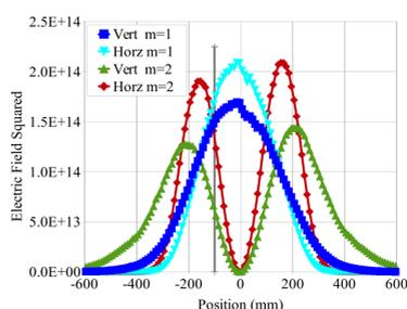
When the round chamber diameter was increased to 95.5 mm, the lowest resonances were confined by the transitions to be mostly within the 560 mm length of the quadrupole magnet. This dimension was used in the final design.
