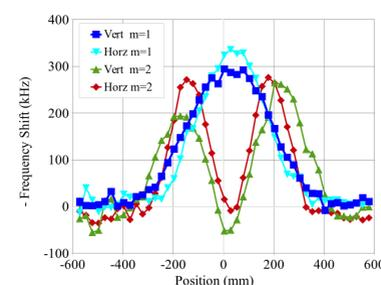
In a bead pull measurement, the shift in resonant frequency is proportional to the square of the resonant electric field at the location of the bead. A bead pull measurement was performed on the fabricated 95.5mm dia. chamber which confirmed the simulation result – that the lowest modes were mostly within the 560 mm length of the quadrupole magnet.
