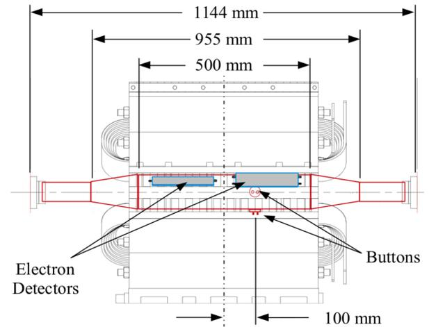
The detector chamber is positioned within a quadrupole magnet. Electron detectors are aligned to one of the pole faces. Beam-position-monitor-style buttons couple to either horizontal or vertical TE<sub>11</sub> modes
