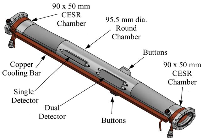
The new chamber supports two independent techniques for measuring electron cloud density: 1) electron detectors using striplines and 2) microwave measurements using beam-position-style button electrodes. The chamber transitions from round beam-pipe in the center to the quasi-rectangular standard CESR cross-section at either end.
