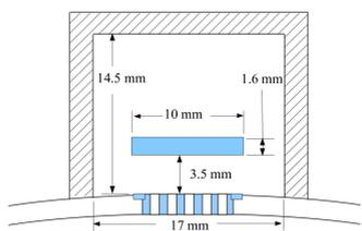
Holes in the beam-pipe wall allow electrons to be collected by the stripline while shielding it from the beam-induced electromagnetic pulse of the beam.
