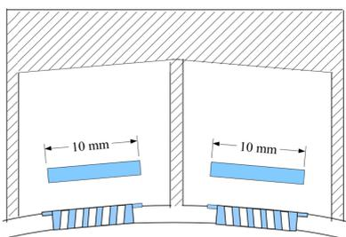
The dual stripline has holes that are angled to follow the magnetic field lines of the quadrupole field. Both the single and dual stripline assemblies are centered on a pole face, but are at different longitudinal positions.
