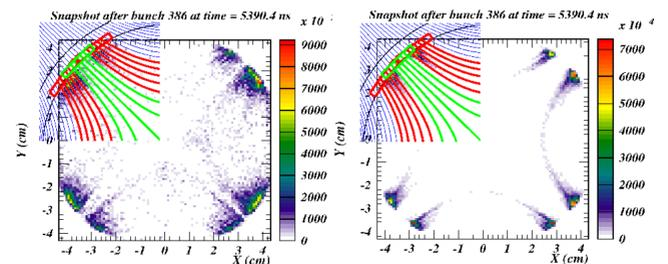
ECLLOUD simulation of the EC density just after the passage of a 20-bunch train of 5.3 GeV positrons with 14 ns spacing shows an increase in the splitting of the cloud near the pole face as the bunch population is increased from  $1.2 \times 10^{11}$  (left) to  $1.3 \times 10^{11}$  particles/bunch (right). The green lines represent electron trajectories through the holes of the single stripline detector; red lines are the trajectories into the dual detector.
