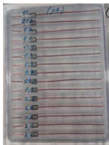
Figure 4: Only 15 feedthroughs out of 1700 pieces are not accepted.
