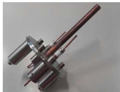
Figure 6: “Head” after welding.
