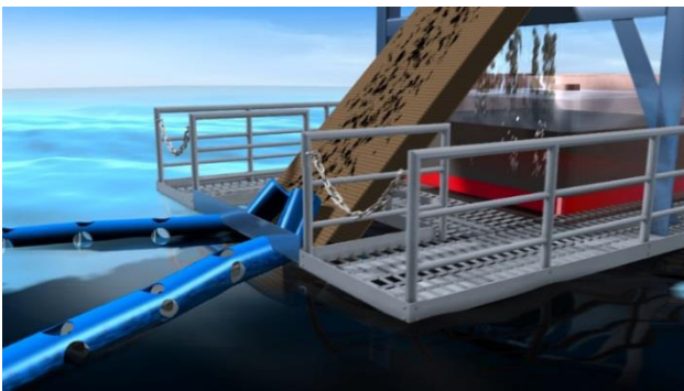
Figure 15: Schematic of collector and separator component of the system.
