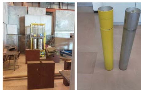
Figure 12: Insulation of icBLM.
