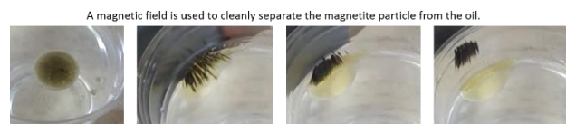
Figure 6: Sequence of images illustrating the magnetic separation of the magnetite particles from the oil using a permanent magnet.
