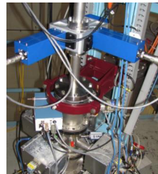
Figure 7: UniBEaM installed at the entrance to pelletron accelerator.
