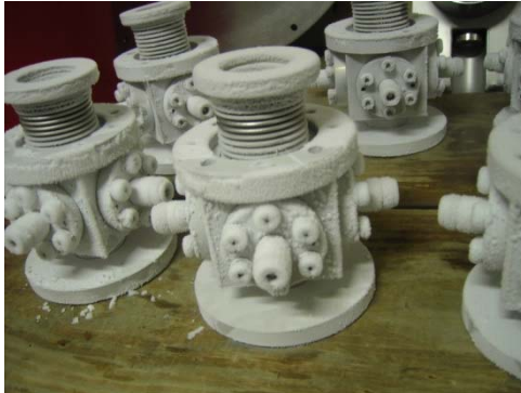
Figure 3: The liquid nitrogen test of the BPM pick-ups.
