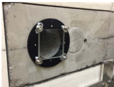
Figure 7: Flat optical window installed on the shielding wall to block the air flow.
