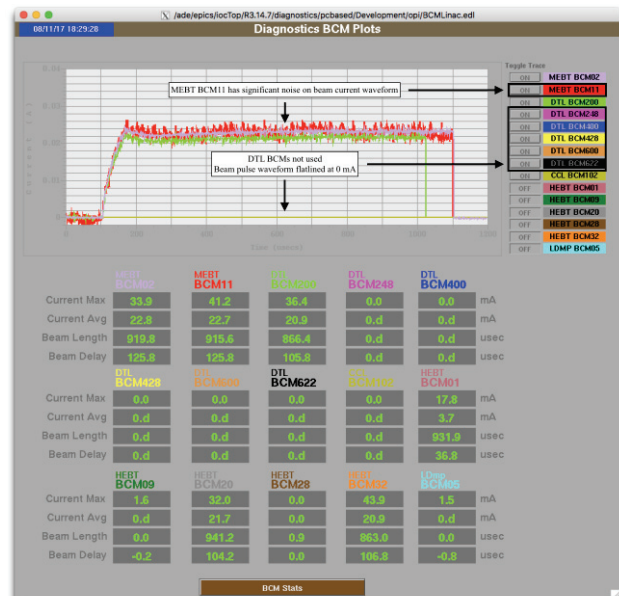
Figure 5: Example BCM waveforms showing a noisy signal in the MEBT, and that DTL BCMs are not used.
