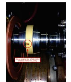
Figure 4: Picture of CCL BCM after being damaged by field emitted electrons.
