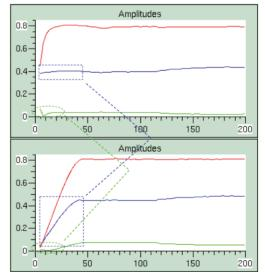
Figure 8: Y-axis is arbitrary FCM field units and x-axis is time in microseconds. Red is cavity field waveform, blue is cavity forward power waveform, green is cavity reflected power waveform. Changing the forward power fill from constant (top image) to a slower linear ramp (bottom image) changed the reflected power structure during the fill and reduced RF faults.
