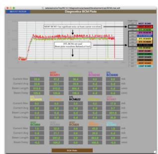
Figure 5: Example BCM waveforms showing a noisy signal in the MEBT, and that DTL BCMs are not used.
