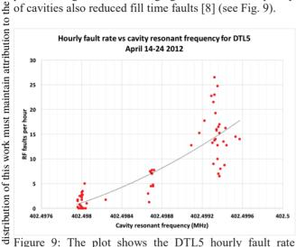
Figure 9: The plot shows the DTL5 hourly fault rate Any versus cavity resonant frequency during a 10 day period in April 2012. Decreasing the cavity frequency from 8 402.500 MHz to 402.498 MHz significantly reduced the 201 fault rate. 0
