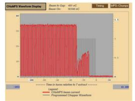
Figure 2: Example of LEBT high voltage malfunction.
