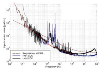
Figure 4: Noise spectrum taken from the FAIR Nb CCC in comparison to a Pb system.
