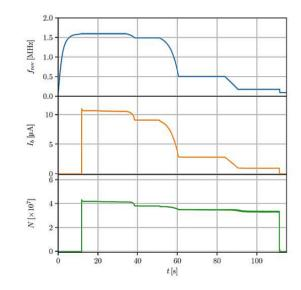
Figure 3: Deceleration cycle of the CERN AD. Revolution frequency (upper), beam intensity measured with CCC (middle) and corresponding particle numbers (lower).
