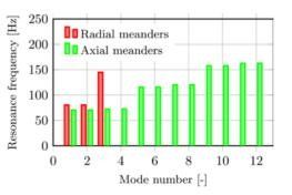
Figure 8: Mechanical eigenfrequencies of radial and axial magnetic shieldings up to 200 Hz. Both shields exhibit a  $-75 \pm 5$  dB attenuation.
