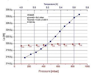
Figure 6: Inductance measurement with the 'anti-cryostat'.
