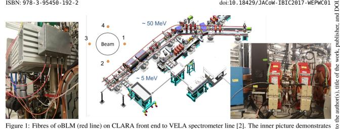
Figure 1: Fibres of oBLM (red line) on CLARA front end to VELA spectrometer line [2]. The inner picture demonstrates the location of four fibres with respect to the beampipe. oBLMs are located at the front end of the beamline therefore the sensors are located upstream. The inner photographs show the oBLM box (left corner) and the fibre locations along the beamline (right corner).
