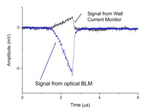
Figure 4: Graph demonstrates measurements which were taken by oBLM (blue signal) and by the Wall Current Monitor (black signal), and their correlation is clear.
