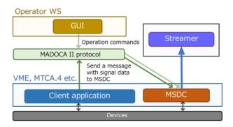
Figure 8: Configuration of MADOCA II data collection processes with MSDC. In this case, the client application prepares signals data and sends a message with signal data to MSDC.
