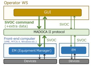
Figure 1: Schematic view of the software framework for messaging controls with MADOCA II.
