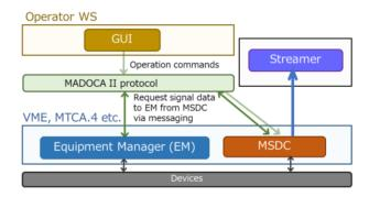
Figure 7: Configuration of MADOCA II data collection processes with MSDC. MSDC fetches signal data from an EM with the messaging commands of MADOCA II.
