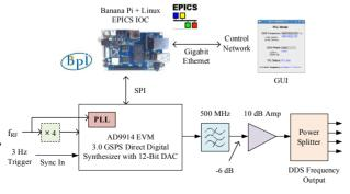
Figure 3: Block diagram of the DDS control.
