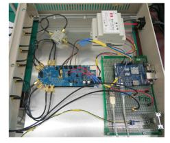
Figure 6: Photo of the frequency divider unit.
