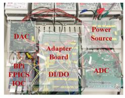
Figure 10: Prototype validation of the corrector power supply control.
