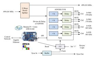
Figure 5: Block diagram of the programmable clock generator.
