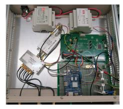
Figure 4: Photo of the DDS signal generator.
