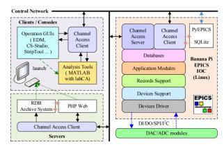
Figure 1: Software architecture of the BPi within EPICS support.
