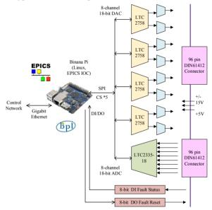
Figure 9: Block diagram of the CPSC-lite.
