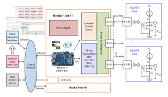
Figure 7: Block diagram of the RadFET readers system.
