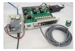
Figure 8: Prototype of the 16 channels RadFET reader with BPi EPICS IOC.
