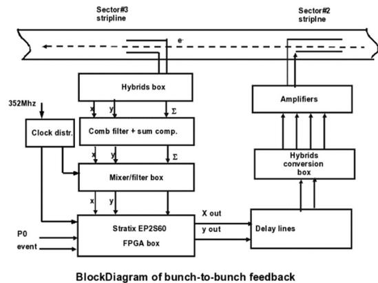
Figure 1: Block diagram of the feedback system.
