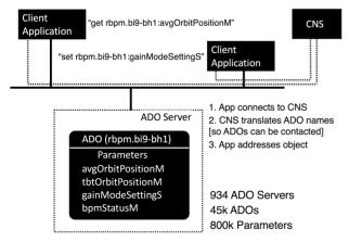
Figure 1: C-AD Controls ADO communication model.
