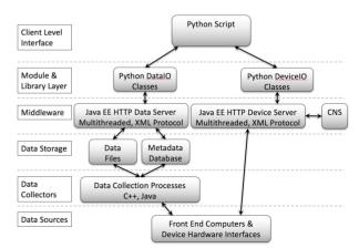
Figure 2: Example of HTTP communications model.
