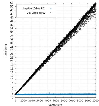
Figure 2: Data Transfer speed: d-bus vs. pipe.
