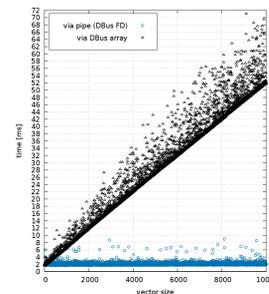
Figure 3: Data Transfer speed with concurrent d-bus users.
