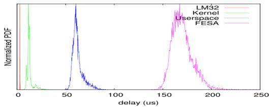
Figure 1: Latency measured by oscilloscope.
