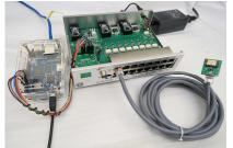
(b) Photo of the prototype 16 channels RadFET reader with BPi EPICS IOC.
