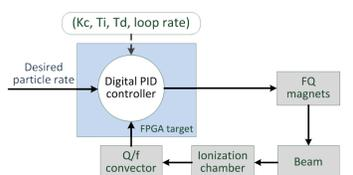
Figure 4: The spill feedback processing
