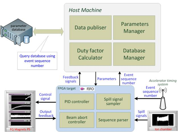
Figure 3: Block diagram of the feedback unit.
