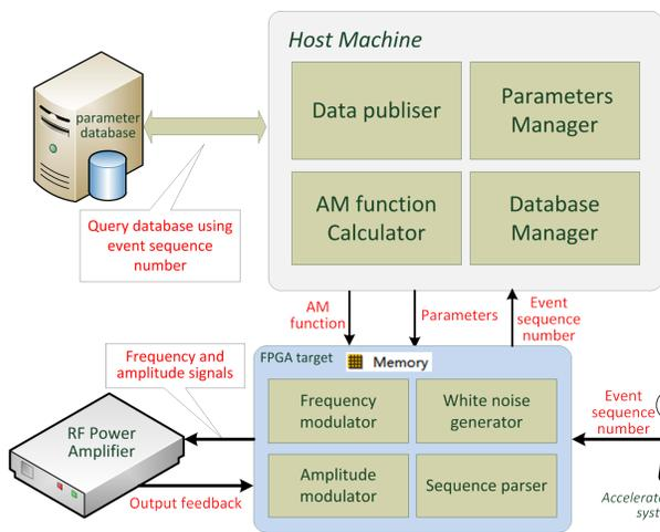
Figure 1: Block diagram of the RF-KO exciter unit
