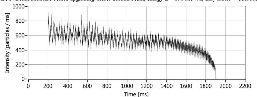
Figure 6: Beam structure without FQ feedback after upgrading. Here: Carbon beam, energy E = 190 MeV/u, duty factor = 89.19%
