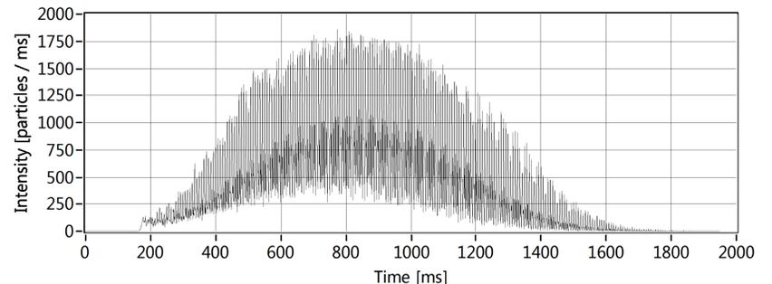
Figure 5: Beam structure before upgrading. Here: Carbon beam, energy E = 190 MeV/u, duty factor = 35.98%
