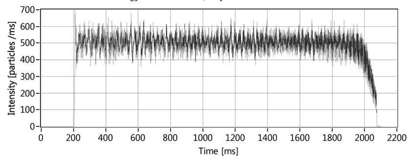
Figure 7: Beam structure with FQ feedback after upgrading. Here: Carbon beam, energy E = 190 MeV/u, duty factor = 92.13%
