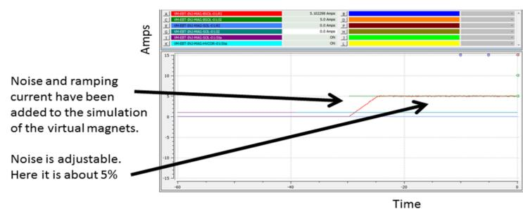
This is an example of a virtual magnet used to test a new Qt GUI striptool running under EPICSQt. The full online model is not needed here and just a basic set of magnet parameters are being simulated. Here the magnet current ramping, interlocks and noise are being generated in the virtual IOC. This tests was useful for rapid application development for CLARA GUIs
