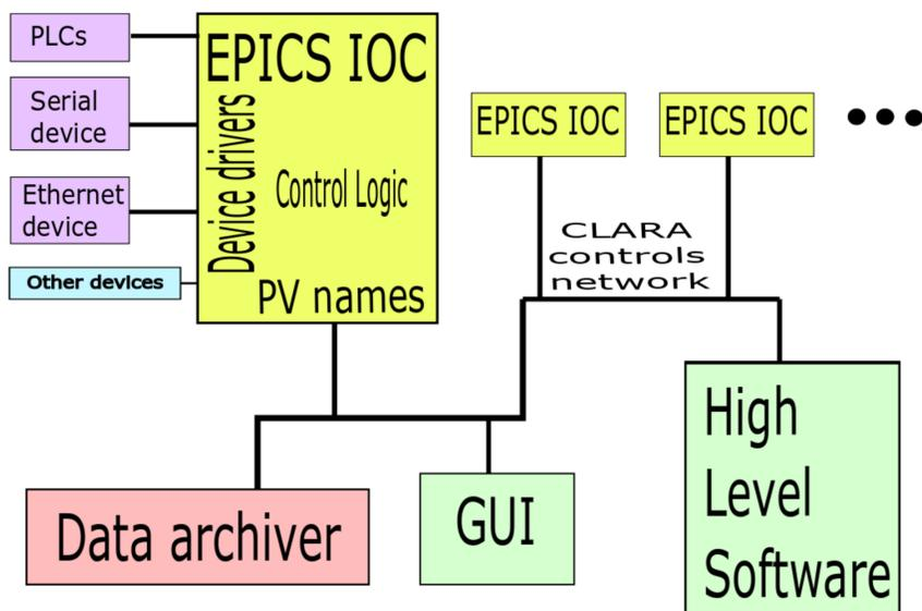
The CLARA technical sub-systems are managed within a distributed control system implemented with the EPICS software toolkit. The core of EPICS are IOCs that provide common controls over a network via Process Variables. A virtual accelerator has been made that simulates CLARA subsystems. The virtual PVs can be used without any particle tracking, providing simple functionality. In the case of magnets; current and interlocks. This mode has been used in the development of GUIs and State Machines.
