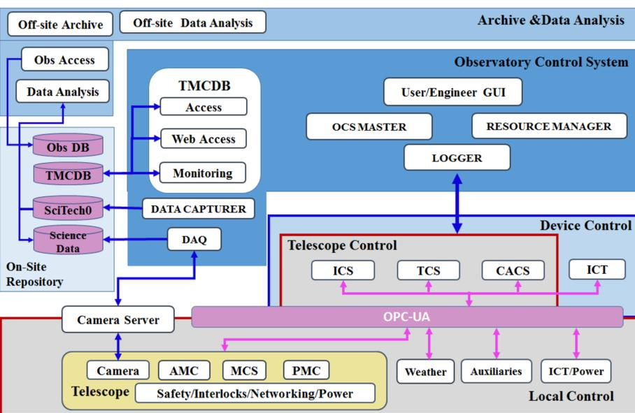
Fig. 1: ASTRI MASS Software Architecture
