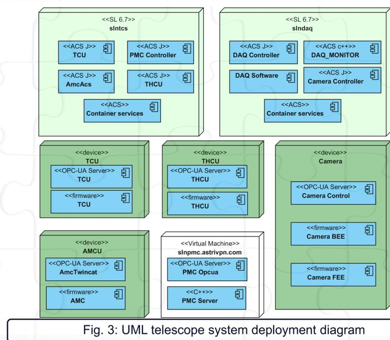
Fig. 3: UML telescope system deployment diagram
