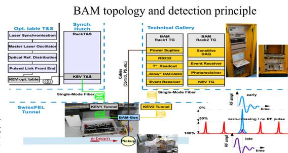
A pulse train from a mode locked laser at 1560 nm and 142.8 MHz repetition rate is sent to the BAM front end ("Box") via length
