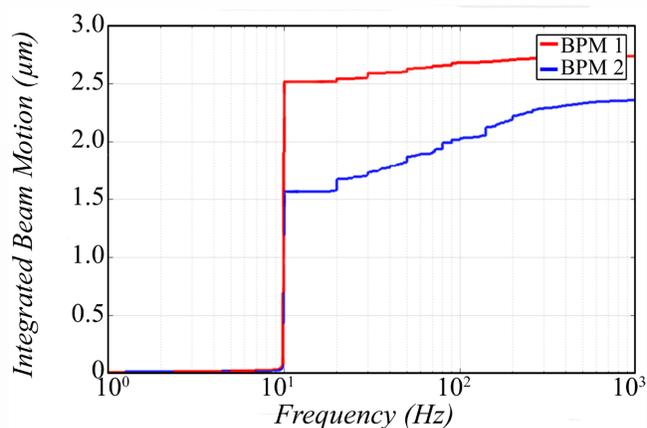
Effect of fast chicane switching on integrated beam noise.
