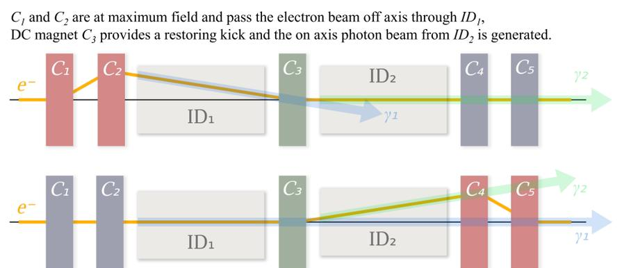
The AC waveform is cycled 180° out of phase between  $\{C_1 C_2\}$  and  $\{C_4 C_5\}$  to provide 10 Hz oscillations between the two on axis trajectories.
