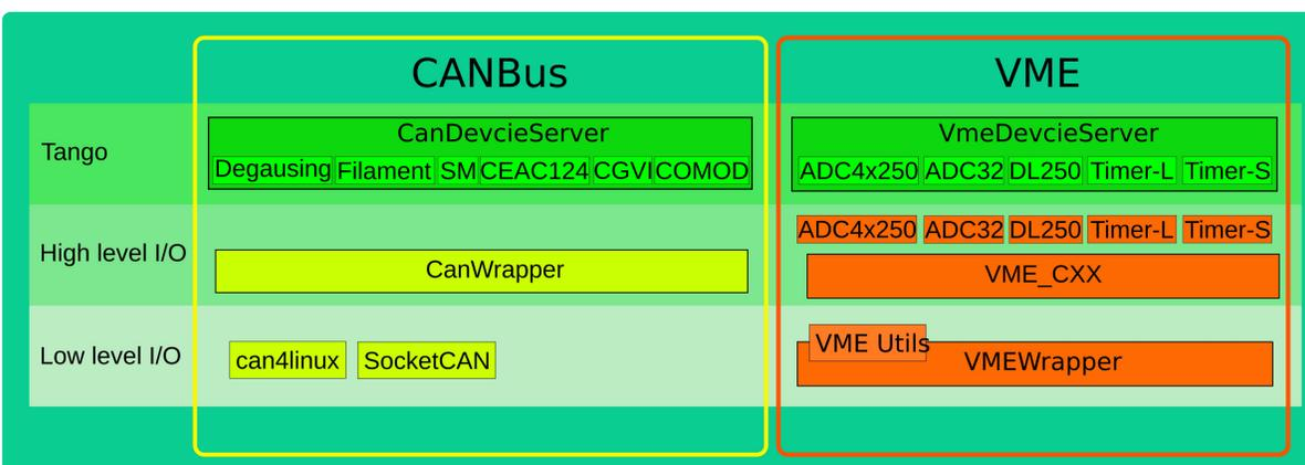
**Low level I/O** layer consists of CANBus driver (can4linux or SocketCAN) and VME wrapper.
