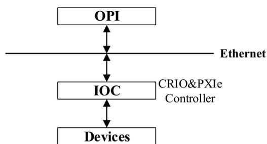
The control System structure is based on EPICS.
