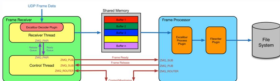
OdinData architecture showing Excalibur use case.
