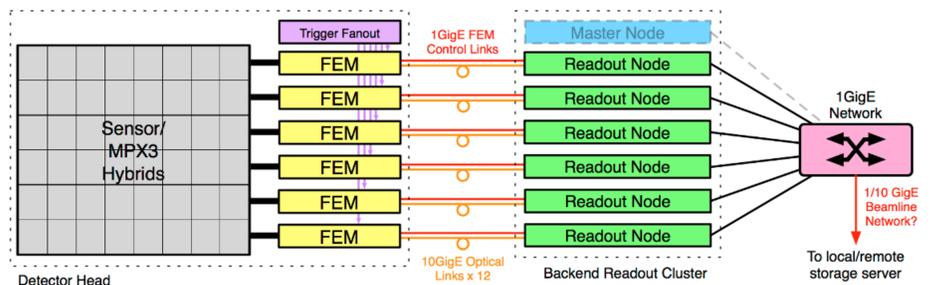
A schematic of the Excalibur 3M system [5].
