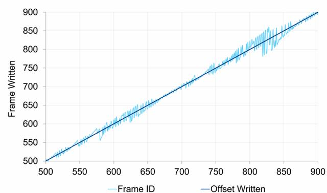
A graph showing the order and offset of frames written during an Eiger acquisition. The Frame ID shows that frames are written out of order, because some nodes fall behind others, while the linear Offset Written proves that the frames are still written to the correct offsets in the HDF5 dataset.
