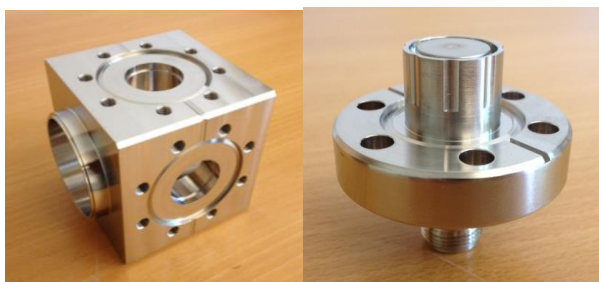
Figure 3: Picture of a prototype 60 mm ESS BPM (left) and the DESY-XFEL type button (right).
