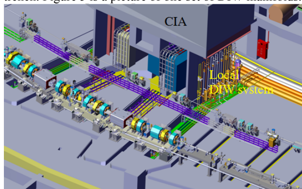
Figure 4: 3D schematic draw of a local DIW system.
