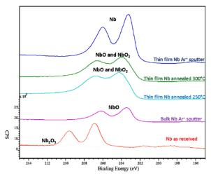
Figure 2: Nb 3d region scan for bulk and thin film as received, sputtered and annealed.
