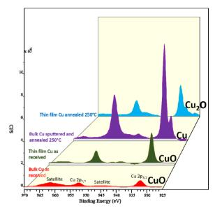
Figure 1: Cu 2p region scan for bulk and thin film as received, sputtered and annealed.
